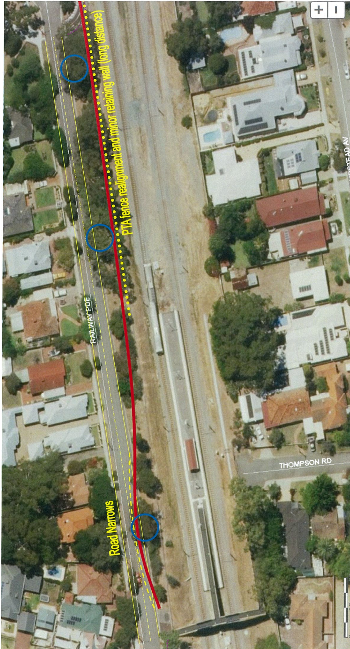
OPTION 1 - Midland PSP alignment along Railway Parade, Bassendean. Narrowing of Railway Parade (one section, west end), PTA fence relocation (mid section to east end) expected long low height retaining wall, no road drainage impact expected, additional vegetation to be planted
